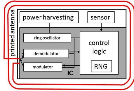
Fig. 4: System architecture of the resource restricted IoT sensor node. The random number generator (RNG) is an inherent part of the circuit logic.
